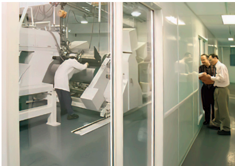
Clear, aliphatic TPU film being made in an 8,000 sf hard-walled white room
