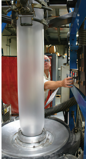
Blown film lab lines can extrude up to 86" (218.4 cm) wide and 1.0 to 12.0 mils thick
