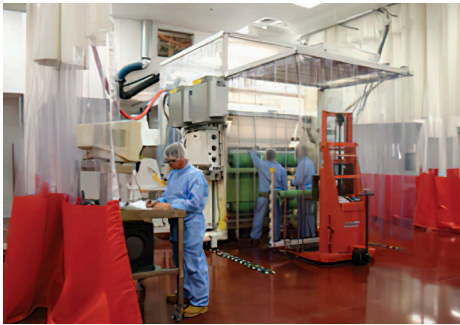
Class-7 soft-walled clean rooms inside an 8,000 square foot hard-walled white room
