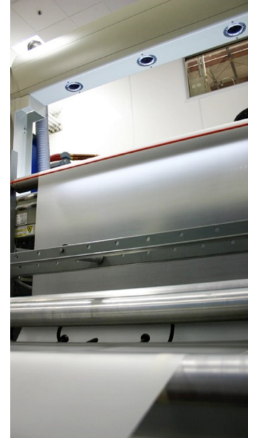
In-line visual camera inspection ensures consistent quality
