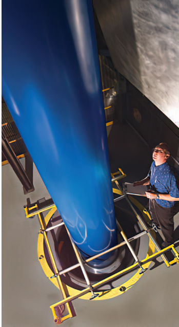
Blown film lab lines can extrude up to 86" (218.4 cm) wide and 1.0 to 12.0 mils thick
