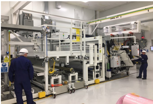
Optically clear aliphatic TPU film is produced in an 8,000 sf hard-walled white room
