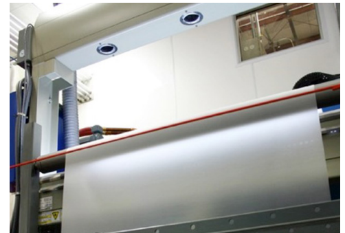
In-line visual camera inspection ensures consistent quality
