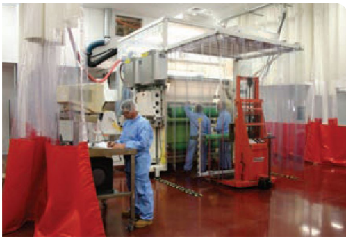
Optically clear aliphatic TPU film is produced in a soft room inside an 8,000 sf hard-walled white room
